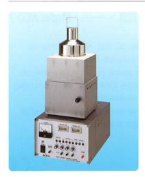
ACR-6 automates the cracking/coking process of Conradson carbon residue test. The microprocessor controlled oven requires less experience to conduct the tedious process and therefore yields more consistent test result.
